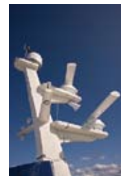
The tri-fold mast drops the waterline height to under 20 feet, allowing passage through New York’s Erie Canal system.
